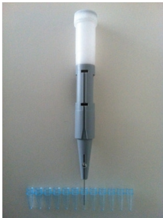
Figure 2 – Single-channel pen-shaped gel cartridge.
